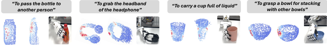
Figure 6: Real-world experimental results. For each task, the left, middle, and right images show the template contact map, the transferred contact map, and the generated dexterous grasp, respectively.
