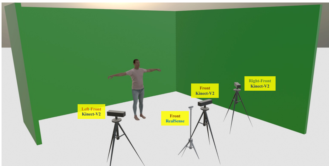
Figure 1: Schematic diagram of our recording studio.
