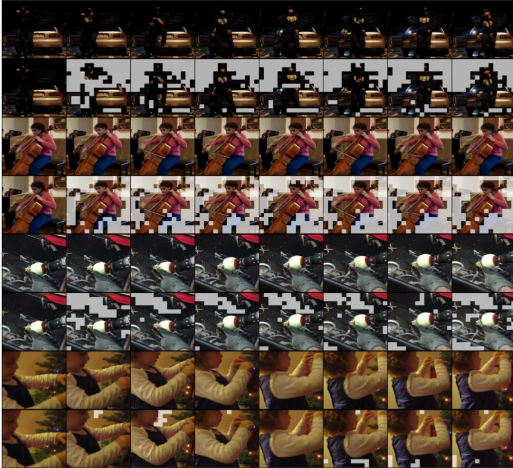
Figure 4: Sample Visualizations. Tokens that are compressed are visualized in gray. RLT retains tokens that change between frames while removing redundant tokens. In the top example, RLT captures the static background, and in the bottom example, due to camera motion and the motion of the girl, almost no tokens are modified. Video visualizations are available at the project page.
