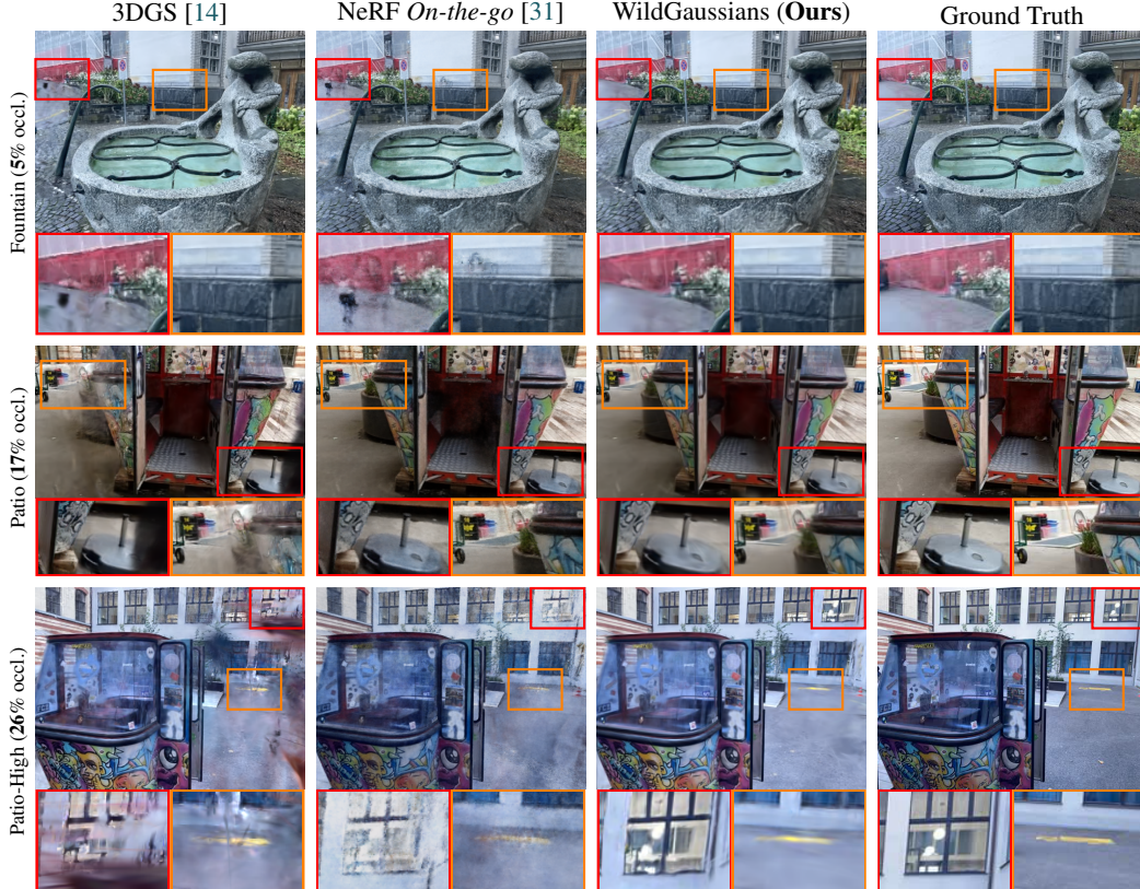
Figure 4: Comparison on NeRF On-the-go Dataset [31] . For both the Fountain and Patio-High scenes, we can see that the baseline methods exhibit different levels of artifacts in the rendering, while our method removes all occluders and shows the best view synthesis results.
