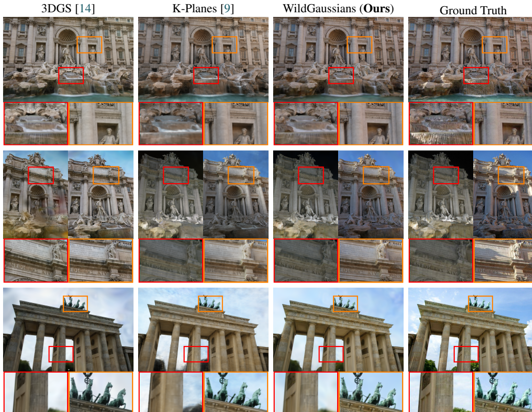
Figure 5: Comparison on the Photo Tourism Dataset [35] . In the first row, note that while none of the methods can represent the reflections and details of the flowing water, 3DGS and WildGaussians can provide at least some details even though there are no multiview constraints on the flowing water. On the second row, notice how 3DGS tries to ‘simulate’ darkness by placing dark - semi-transparent Gaussians in front of the cameras. For WildGaussians, the text on the building is legible. WildGaussians is able to recover fine details in the last row.
