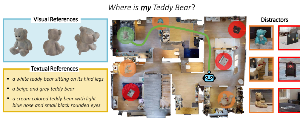
Figure 1: We introduce the PIN task, where the agent is asked to navigate toward a personalized object instance using multimodal references and distinguish it from distractors ( i.e. , other objects of the same category as the target or of other categories). The target object, same category distractors, and other distractors are circled, respectively, in green, orange, and red. The total number of available objects in the dataset is 338, corresponding to different instances of 18 object categories.
