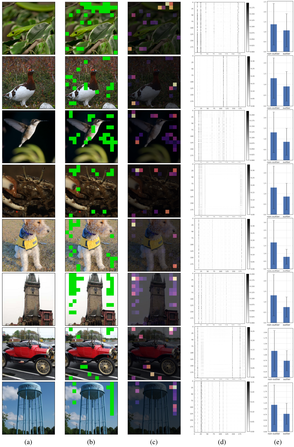
Figure 17: A summary of our outlier analysis for ViT demonstrated on a random subset from ImageNet validation set. (a) An input image. (b) Outliers in the output of layer #11. (c) Cumulative attention weight spent on every patch (matrix of attention probabilities summed over rows) in the attention head #1, in the next layer #12. (d) A corresponding matrix of attention probabilities. (e) An average magnitude of values ( V ) for outlier and non-outlier patches.
