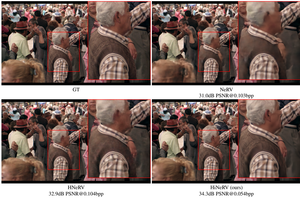
Figure 7: Comparison between the output of NeRV, HNeRV and HiNeRV with the videoSRC14 sequence from the MCL-JCV dataset [25].
