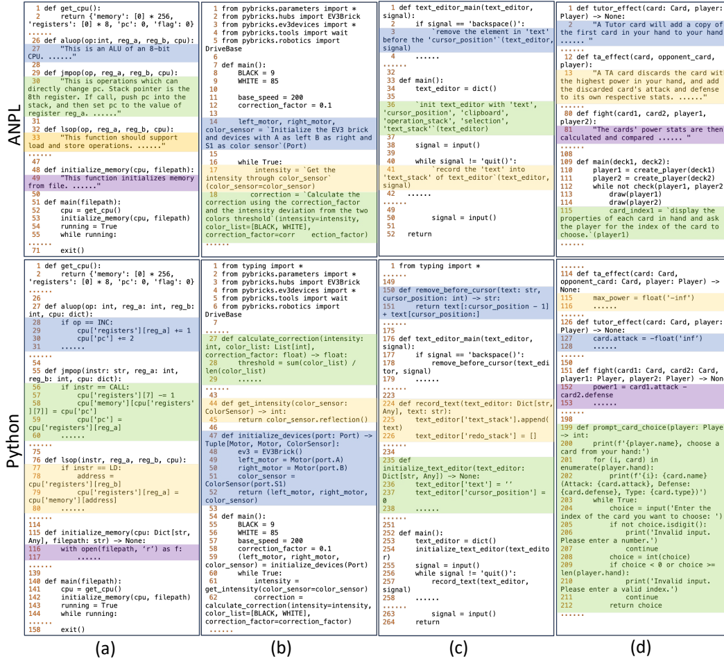
Figure 21: The ANPL and Python code of four projects: (a) LS-8 CPU (b) a robot controller (c) a text editor (d) a naive MAGIC. We present part of the code and mark the ANPL code and its corresponding Python code with the same background color.
