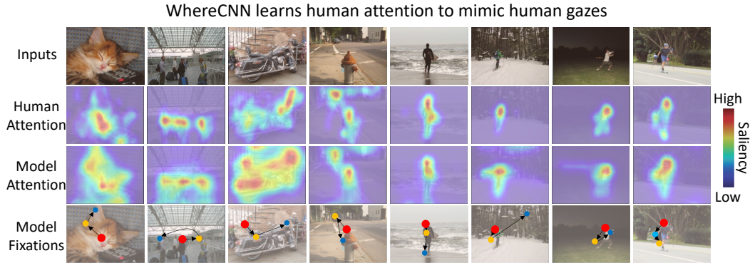
Figure 2: Saliency prediction. Given an image (1st row), WhereCNN generates a saliency map (3rd row) similar to the map of human attention (2nd row). Sampling this saliency map generates a sequence of fixations (as red/orange/blue circles in the 4th row) similar to human saccadic eye movements (not shown).
