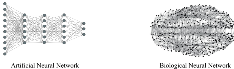
Figure 1: Difference in topology between an artificial neural network (left), and a sketch of a network of structural connections that link distinct neural elements in a brain (right) [26].
