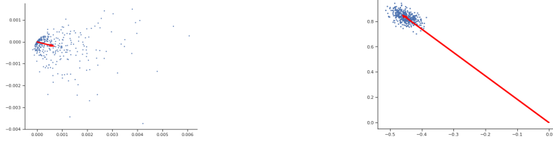
Figure 1: 2-d PCA under the Gaussian data from Remark 3.4 (left) shows that the average gradient (red arrow) is smaller than the range of the minibatch of 400 gradients (blue dots). Under Example 4.1 (right), the range can be made arbitrarily smaller than the average gradient.
