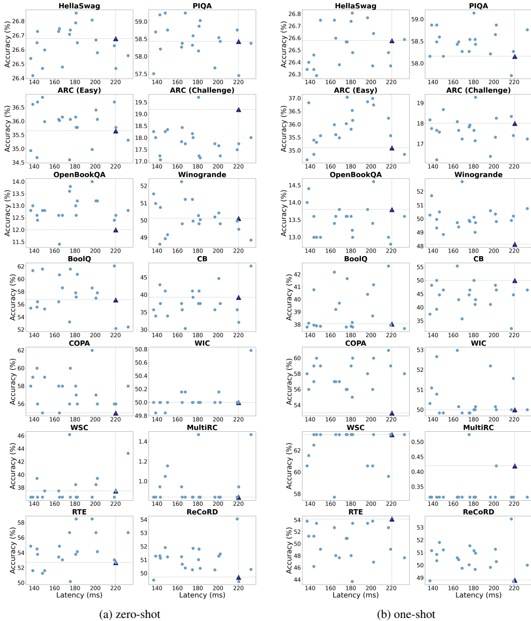
Figure 17: LTS Pareto-frontier models (dots) achieve a higher zero and one-shot accuracy with lower latency compared to the hand-designed OPT-350M model (triangle). Latency is measured on an A6000 NVIDIA GPU. Architectural parameters for all models shown here are detailed in Appendix I.
