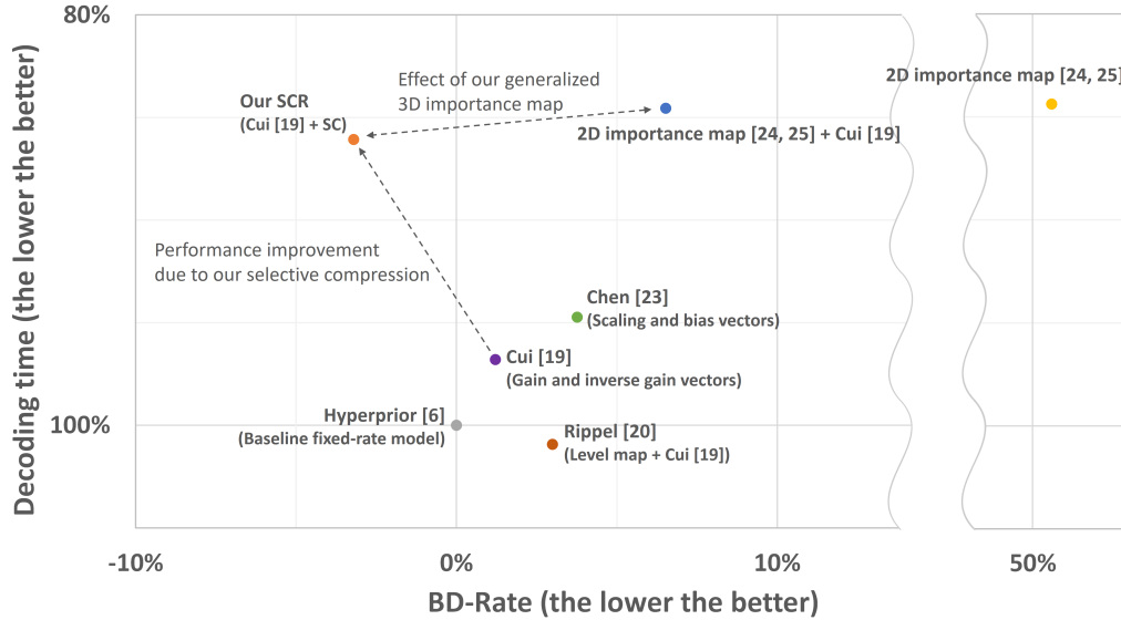
Figure 13: Comparison results of the various variable-rate image compression methods in terms of the coding efficiency and decoding time. For the same condition of comparison, we reproduced these variable-rate methods on the same base architecture, Hyperprior [6]. The PSNR BD-rate values are measured using four (first, fourth, sixth, and eighth) compression points. "SC" denotes the proposed selective compression.
