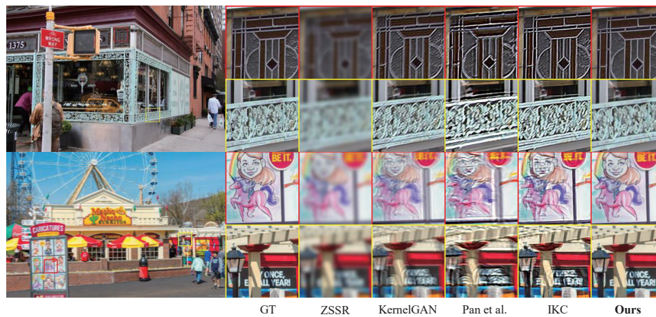
Figure 5: 2\times Blind SR results for LR degraded with unknown motion kernel from Flicker2K.
