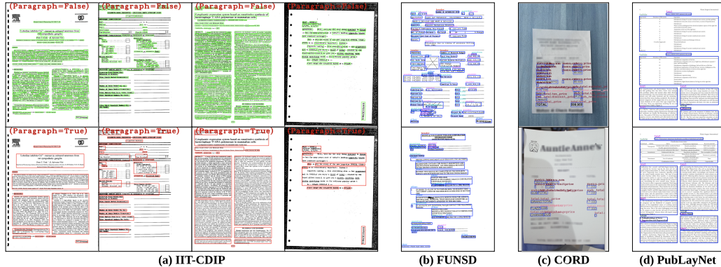
Figure 3: Document image samples. The boxes in red/green are OCR bounding boxes obtained with/without paragraph mode, while the boxes in blue are officially-provided bounding boxes.
