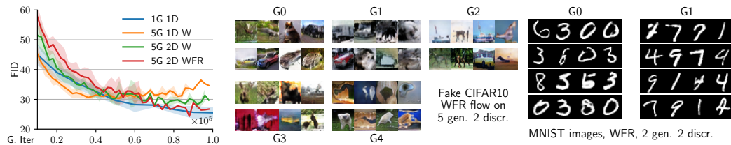
Figure 3: Training mixtures of GANs over CIFAR10. We compare the algorithm that updates the mixture weights and parameters (WFR-DA flow) with the algorithm that only updates parameters (W-DA flow). Using several discriminators and a WFR-DA flow brings more stable convergence. Each generator tends to specialize in a type of images. Errors bars show variance across 5 runs.
