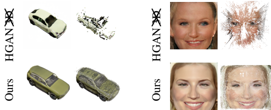
Figure 7: 3D Reconstruction from synthesized images at resolution 256^2 . Each pair shows one of the generated images and the 3D reconstruction from COLMAP [60].
