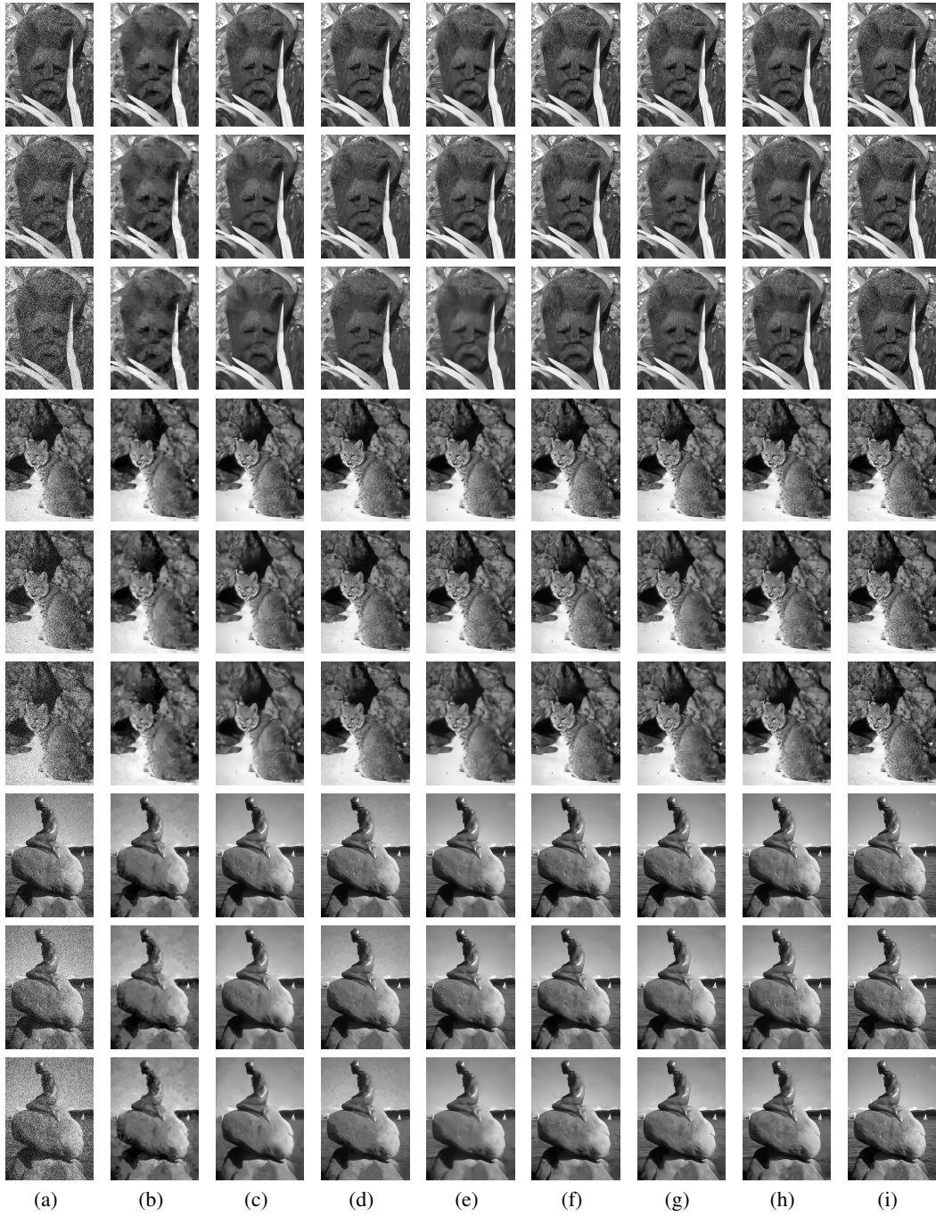
Figure 5: The qualitative comparisons on the denoising task using BSD500. From the top to the bottom for each image, the noise levels are \sigma = 30, 50, 70 . From the left to the right are Input, BM3D [1], RED [9], WNNM [3], NLRN [6], DuRN-P [7], N3Net [10], CLEARER, and Ground truth.
