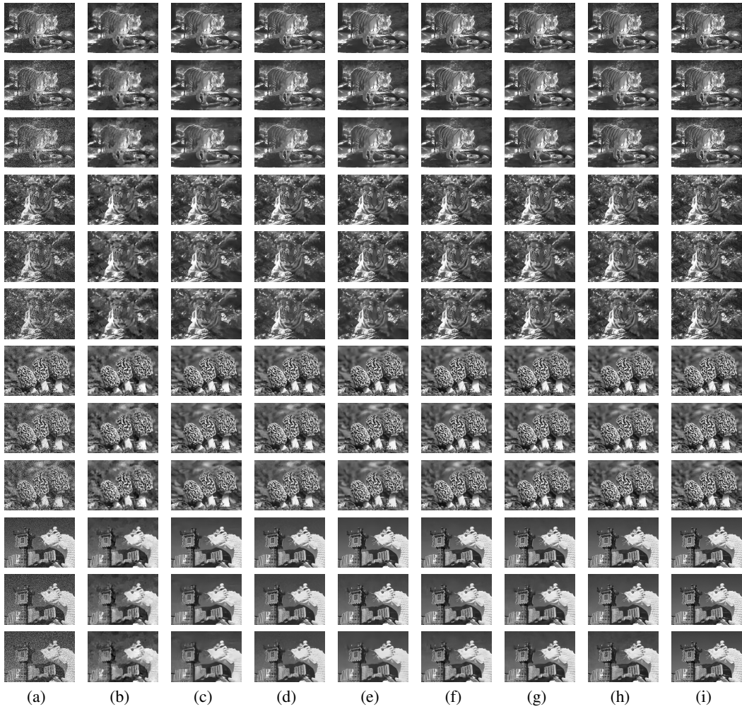
Figure 6: The qualitative comparisons on denoising task using BSD500. The noise levels for each image from the top to the bottom are \sigma = 30, 50, 70 . From the left to the right are Input, BM3D [1], RED [9], WNNM [3], NLRN [6], DuRN-P [7], N3Net [10], CLEARER, and Ground truth.
