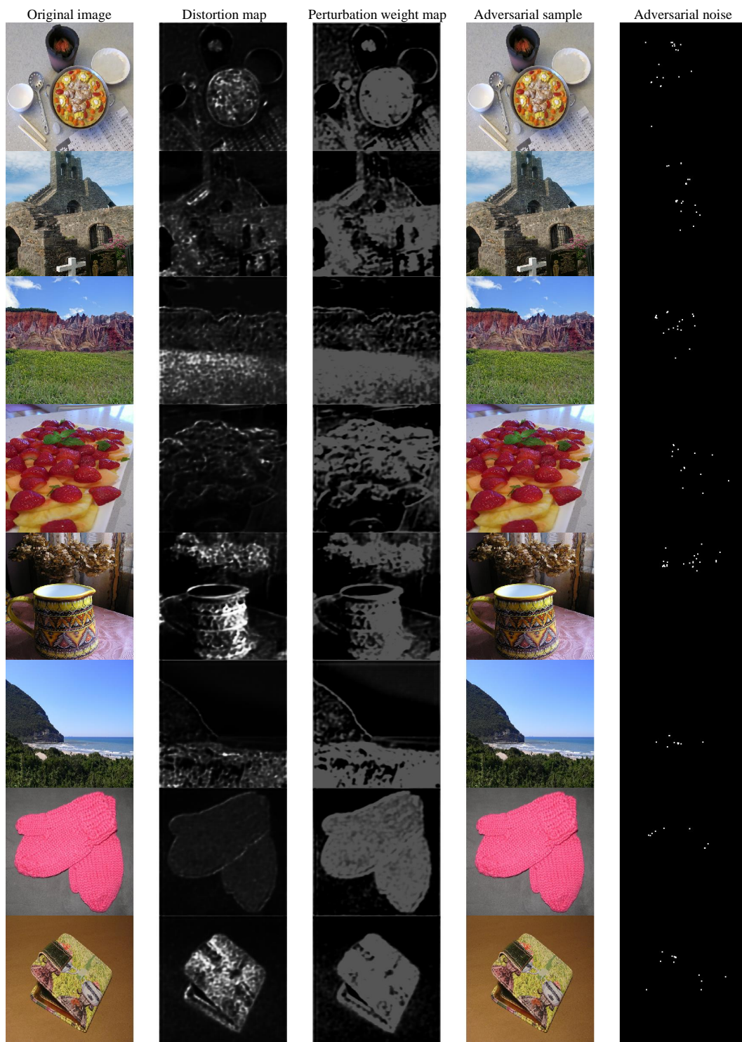
Figure 2: More visual results of our GreedyFool with \epsilon = 255 on ImageNet dataset. Besides the adversarial sample, we also show its corresponding distortion map \varrho , perturbation weight map \mathbf{p} , and adversarial noise (We enlarge the noise size to 2 \times 2 pixels for more visible.)
