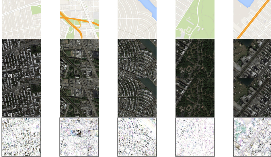
Figure 9: Image synthesis: from label maps to fake satellite images. Row 1: Original label maps, Row 2: Satellite images generated by the original generator, Row 3: Satellite images generated by the pruned generator, Row 4: Residual difference between generated images in Row 2 and 3 amplified by 10x.
