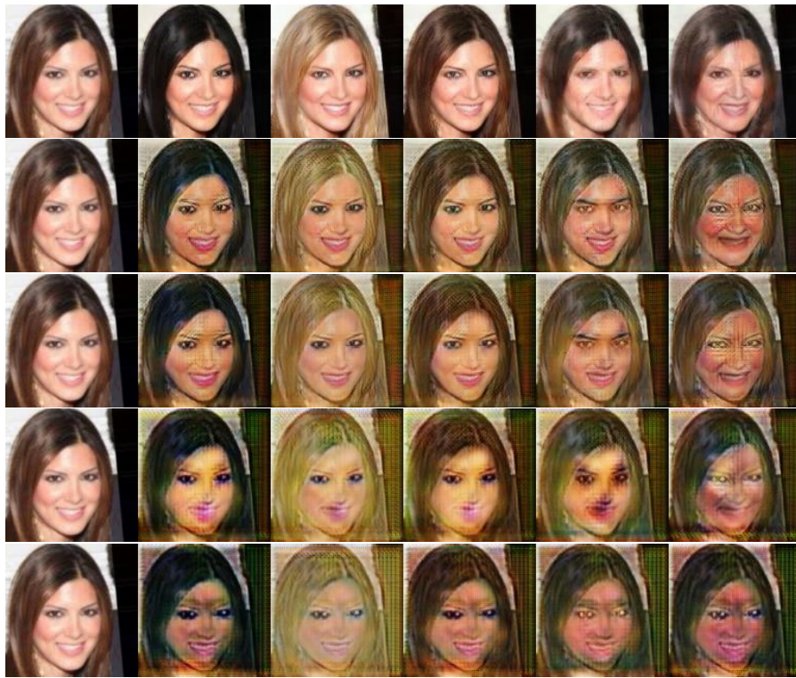
Figure 34: Image-to-image translation example 2: filter pruning to different sparsities. Row 1: Baseline generator output. Rows 2-5: Facial attribute translated images by generators pruned to sparsities of 25%, 50%, 75%, 90%.
