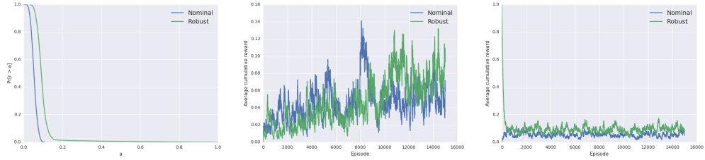
Figure 5: Tail distribution and cumulative rewards during transient and stationary phase of robust vs nominal Q-learning on FrozenLake-v0 with p = 0.1 .
