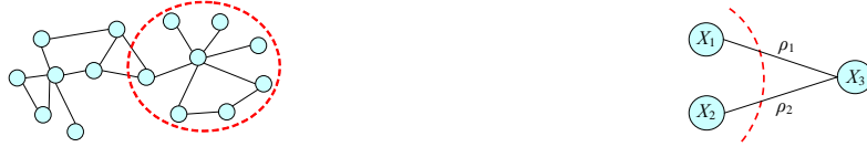
Figure 1: Left: A simple subnetwork of interest, marked with the dotted circle. Right: Illustration of the Neumann random walk, the dotted curve indicates the boundary of the subnetwork.
