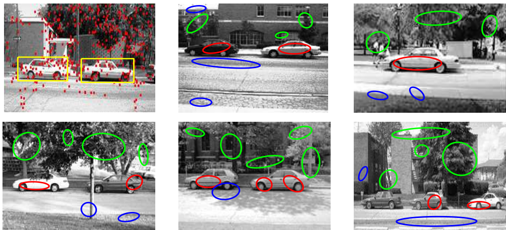
Figure 3: The left most plot on the first row shows the locations of detected patches and the bounding boxes in one of the annotated images. The remaining five plots show examples of detections and localizations of the three most dominant features (including the car-category) in five non-annotated images.
