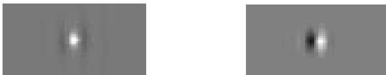
Fig. 3: The measured RF profile of the EVEN and ODD symmetric filters at the center pixel.
