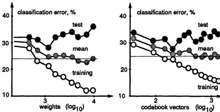
**Figure 3:** a) Measured classification errors for neural networks with increasing number of weights (capacity). The mean value between the test and training error estimates the performance of the given classifier trained with unlimited data. b) Measured classification errors for LVQ classifiers with increasing number of codebook vectors.
