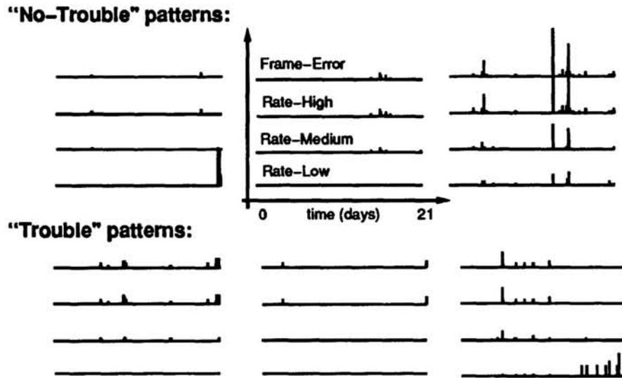
**Figure 2:** Errors as function of time. The 3 top patterns are members of the "No-Trouble" class. The 3 bottom ones are members of the "Trouble" class. Errors are here plotted as mean values over hours.
