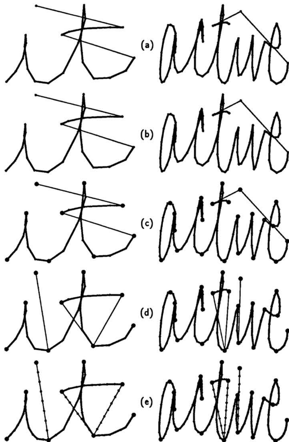
Figure 1: The five principal stages of preprocessing: (a) The original data, x, y values sampled every 10mS . (b) The slant is normalized through a shear transformation; (c) Stroke boundaries are determined at points where y velocity equals 0 or pen-up or pen-down events occur; (d) Delayed strokes are reordered and associated with corresponding strokes of the same letters; (e) Each stroke is resampled in space to correspond to exactly 8 points. Note pen-down strokes are shown as thick lines, pen-up strokes as thin lines.
