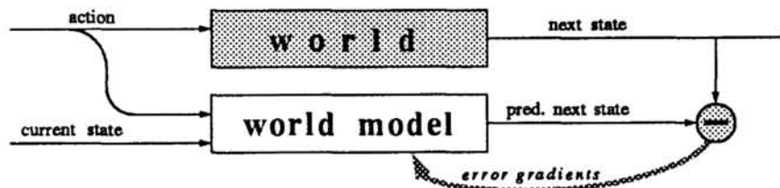
Figure 1: The training of the model network is a system identification task. Weights and biases of the network are estimated by gradient descent using the backpropagation algorithm.
