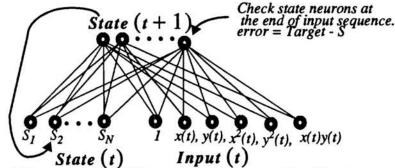
Fig.2 Recurrent Neural Network for Trajectory Classification
