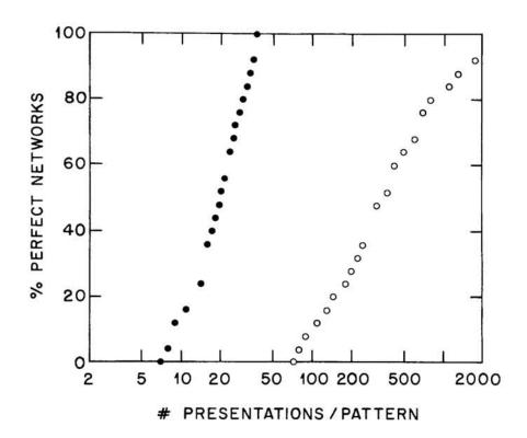
$\underline{\text{Fig. 5}}$ . Learning curves for a symmetry detection network with 4 input units and one hidden unit (deterministic Boltzmann learning,  $\eta = 1$ , discrete  $\pm 1$  units, initial weights random, weights changed after every learning example). Full circles: symmetry-adapted weights; open circles: arbitrary weights, weight randomization (p = 0.015).
