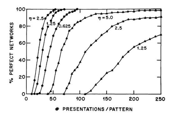
Fig. 4. Learning curves for an XOR-network with three hidden units (backpropagation, initial weights random, weight changes accumulated over all 4 input/output cases). Circles: continuous ±1 units; triangles: continuous 0,1 units.
