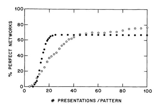
Fig. 1. Learning curves for an XOR-network with one hidden unit (deterministic Boltzmann learning, discrete ±1 units, initial weights zero). Full circles: weights changed after every learning example; open circles: weight changes accumulated over 4 learning examples.
