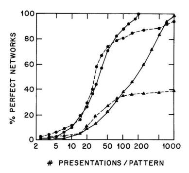
$\underline{Fig.~2}$ . Learning curves for an XOR-network with one hidden unit (deterministic Boltzmann learning, initial weights random, weight changes accumulated over 5 learning examples). Circles: discrete ±1 units,  $\eta$  = 1; triangles: discrete 0,1 units,  $\eta$  = 0.1; broken curves: without weight randomization; solid curves: with weight randomization (p = 0.025).
